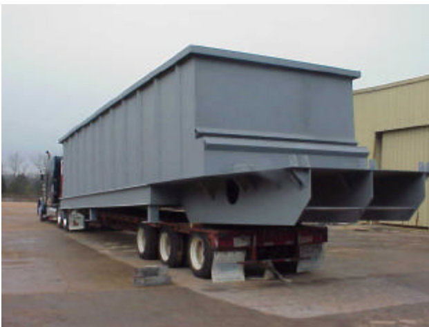
Moss wedge floor being shipped to a Midwest jobsite
